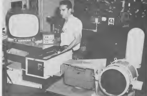
INSTRUMENTMAN HALLEY is shown with the receiver, control, camera and signal light in the shop. The camera and light rotate as one unit so that the light is always directed at the object sighted by the camera. REPARADOR DI instrumento Halley ta para banda di e aparato receptor, control, camera y luz di senjal den shop. E camera cu e luz ta drentu manera un solo unidad, asina ta cu e luz ta tur ora dirigi riba e obheto cu e camera ta mira.
